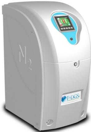
Nitrogen is produced by pressure swing adsorption (PSA) to remove oxygen, carbon dioxide and water from compressed air and purified air is produced by using an activated alumina column.
