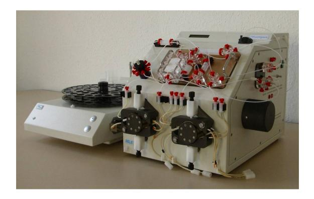
The **FIAcompact** Cyanid-Analyzer determines cyanide in water, eluates and soil extracts acc. to DIN EN ISO 14403.
