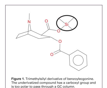
The second reason is to increase the molecular weight of very volatile drugs. This derivatization results in a more complex mass spectrum that improves the selectivity for that particular drug. When derivatizing drugs for GC/MS analysis, the spectrum of the resulting compounds should contain at least three ions that are unique to that analyte and not a result of the matrix.
