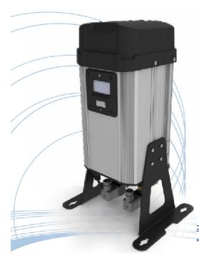
The CO2 adsorption dryers purifier compressed air to deliver a continuous supply of clean, dry (-70 °C pdp) and CO2 free (<1 ppm) purge gas. CO2 adsorption dryers replace high pressure oxygen or nitrogen gas cylinders and are ideal for numerous applications including FT-IR (Fourier transform infrared) purge, TOC purge, NMR, GC flame gas and laser purging.
