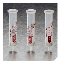
CLEAN SCREEN XCEL® solid phase extraction columns are designed to reduce the number of steps in the extraction. The result is a column that reduces sample prep times and minimizes the amount of solvent necessary. Additional advantages include reduced sample size and improved cleanliness and recovery.
