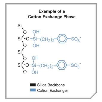
This sorbent is composed of a silica backbone bonded with carbon chains terminated by a negatively or positively charged functional group. Ion exchange interactions occur between a sorbent that carries a charge and a compound of opposite charge.
